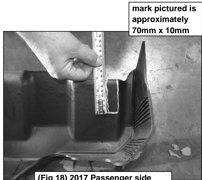
(Fig 18) 2017 Passenger side DEF cover marked for trimming
